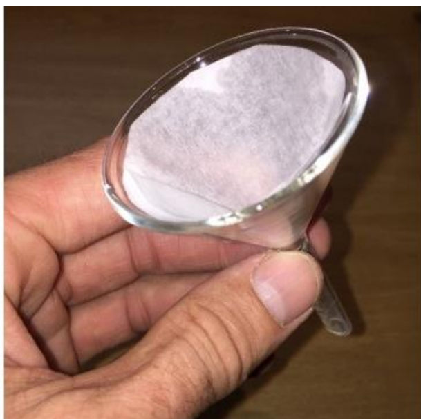
Figure 1.24. Opening the paper up between the folds gives the required filter paper funnel.
