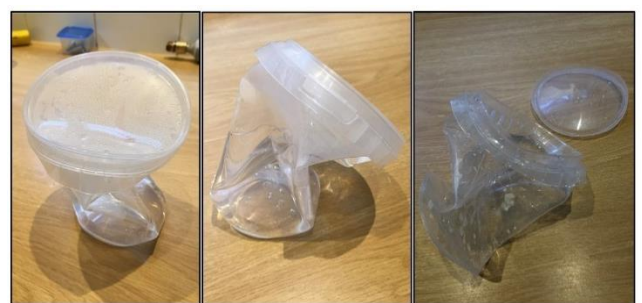
Figure 1.6. Successive collapse of a sealed polypropylene tub during cooling once they have been removed from the autoclave.
